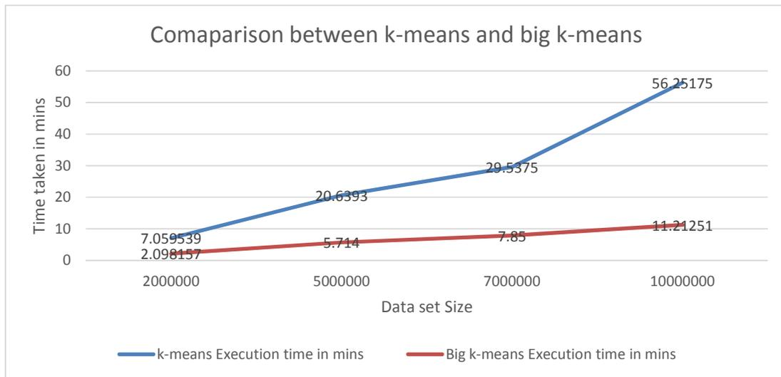
**Fig. 5. Execution time of the k means and big K means according to the size of the dataset**
